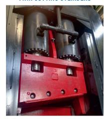
Shears with a twin-cylinder construction create a more balanced and even cutting force which reduces friction on the side walls and guides, ensuring a longer working life with less downtime.
